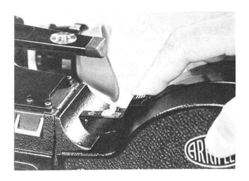
When mounting a magazine, first engage the hinge pin from above into the locating guide (36) on the camera. Then swing the magazine downwards until it clicks into the locking device. When the magazine is seated, flip the safety lock (35) to the "lock" position. Before running the camera, depress the red "test" knob (30) so that the film transport can safely engage the perforation.
