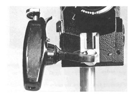
The universal hand grip is the most useful and adaptable of the three grips available. All camera controls can be operated right from the grip, and the grip can be positioned to either the right or the left hand side of the camera. It is mounted to the centrally located accessory shoe (19) on the front of the camera. No cable connections are needed.
