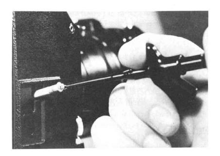
The start mark lamps in the 16 SR are operated below their rated voltage. They should normally have a service life of several hundred hours. Therefore, if a lamp has burned out, consider checking your power supply to see if it is properly rated for the camera.
