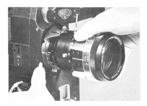
To remove lenses with ARRI steel bayonet mounts, depress the lens release button (58). Then rotate the lens counterclockwise and pull it out of the camera flange.
