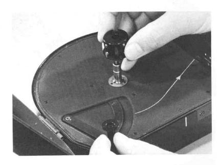
When using film on a plastic core, simply slide it onto the magazine core adapter so that the film unwinds counterclockwise, emulsion in, in the direction of the arrow.
