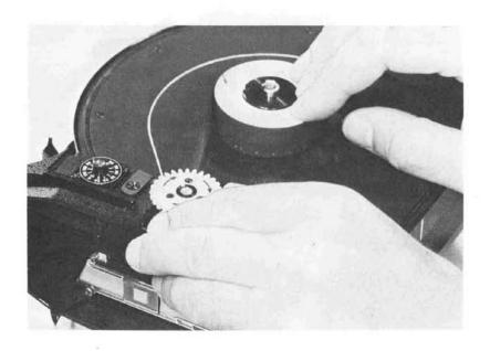
When using daylight spools on the take-up side, remove the core adapter by pressing to the side the button in the centre of the shaft. Engage the film in the slot of the spool and wind a few turns clockwise. Then put the spool on the take-up shaft and tighten the film. The guide arm remains latched away from the spool!
