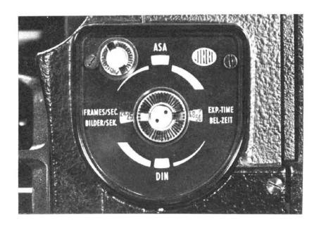
The technical parameters of the exposure meter are unchanged. The light is measured behind the lens in the reflex finder system without the need for semireflecting surfaces between the lens and the film. The measuring area is one third of the total image area, centre weighted.
