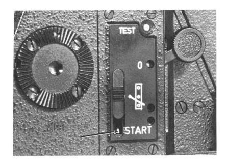
The slow speed electronic inching system can be activated by depressing the small red button marked "test" (30).
