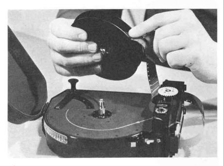
The final step in loading is to slide the film loop under the four retaining hooks, then distribute the film until each side of the loop is of equal size.
