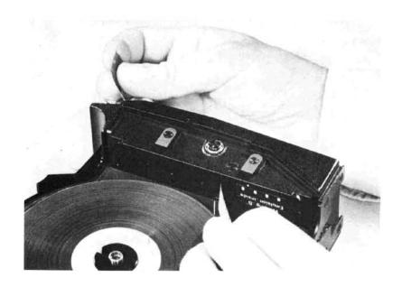
In pushing the film through these guide channels, very little resistance should be felt. If the film does not feed through freely, do not force it! Pull it back out, be sure the loading end is undamaged and start the procedure again.
