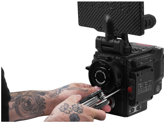
Figure: Remove the OLPF Module
