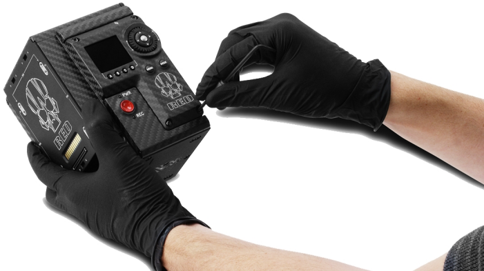
Figure: Reinstall the Side Module/Panel
