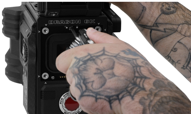
Figure: Turn the Lock Counter-Clockwise
