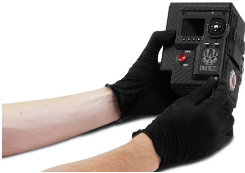
Figure: Remove the Side Module/Panel
