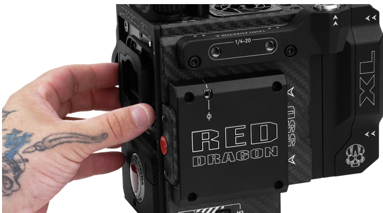
Figure: Install the New OLPF Module
