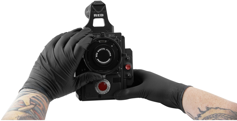
Figure: Turn Locking Ring Counter-Clockwise
