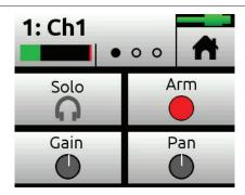
Are you working with a stereo source—a keyboard or stereo mic perhaps? To make it easy to adjust these types of sources, the MixPre-6 offers linking of channel pairs 1-2, 3-4, and 5-6.
