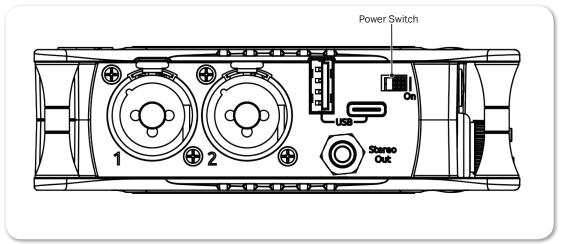
To preserve battery power, USB-C power sources take priority over batteries if both are connected with one exception - if the USB-C power source does not meet the full power requirements of the MixPre-6, you can choose to power from battery or continue to power from USB-C. We have designed the MixPre-6 so that even with an under powered USB-C source, you will still be able to use
