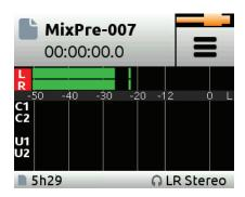
Switching between the three main meter views is easy—just touch the meters and cycle through the different views. The meters will show not only signal levels, but also the current arm status of each track for the recorder and limiting activity for L,R and each channel.
