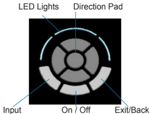
Both the keypad and remote can be used to navigate through the menus. The Main Menu Navigation on the remote functions exactly the same as the directional pad on the P300 unit.
