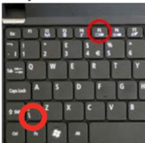
Press function & “F5” to instruct the computer to enable multiple displays. You can also press Windows+P to toggle through display settings.
